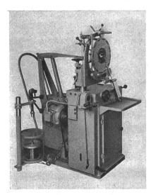
Fig. 2 Statorwickelmaschine
