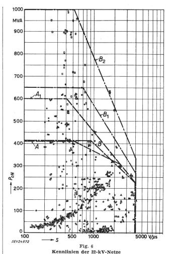
A System A:  $P \le 420$  MVA;  $A_1$  System A:  $P \le 600$  MVA; B System B:  $P \le 420$  MVA;  $B_1$  System B:  $P \le 650$  MVA;  $B_2$  System B:  $P \le 1000$  MVA
