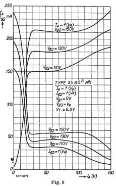
Anode and screen-grid currents as function of the anode-voltage of a specially developed laboratory sample tetrode
