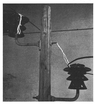
${\bf Fig.~9} \\ {\bf 50\text{-}\%\text{-}Stoss\"{u}berschlag}, \ -{\bf 390~kV} \ ({\rm kleinster~Wert})$
