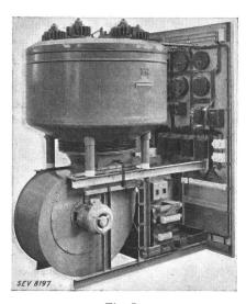
Fig. 7. Mutator-Bloc. 1600 A, 600 V. (Brown Boveri.)
