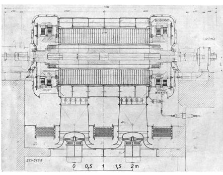
Fig. 7. Drehstromgenerator. 37 500 kVA, 22 000 V, 3000 (Brown Boveri.)
