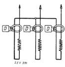
Fig. 7. Self balanced protection.
