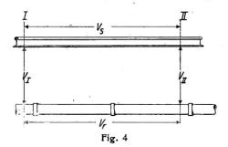
$$V_s + V_{II} + V_r + V_I = 0 (2)$$
