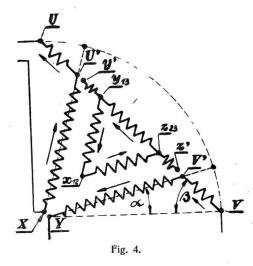
$I_2^2 r_2 \frac{2 + (\sqrt{3} - 1)(\sqrt{6} + 1)}{3} = 2,78 I_3^2 r_2$   $I_3 = I_2 \sqrt{\frac{1,5}{2,78}} = \sim 0,728 I_2$ (17)
