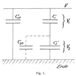
$$\frac{V_1}{V_2} = \frac{C_2}{C_1}$$
