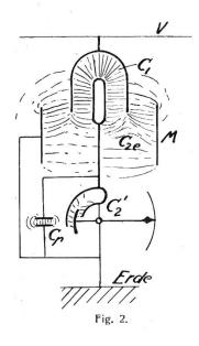
$$V_2 = V_1 \frac{C_1}{C_2}$$
