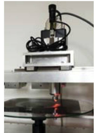
The VisualAudio system captures damaged records in images and reproduces them as audio. (photo: Miriam Bolliger Cavaglieri).
