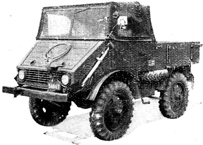
Schlepper Unimog, 4×4, 1 t
