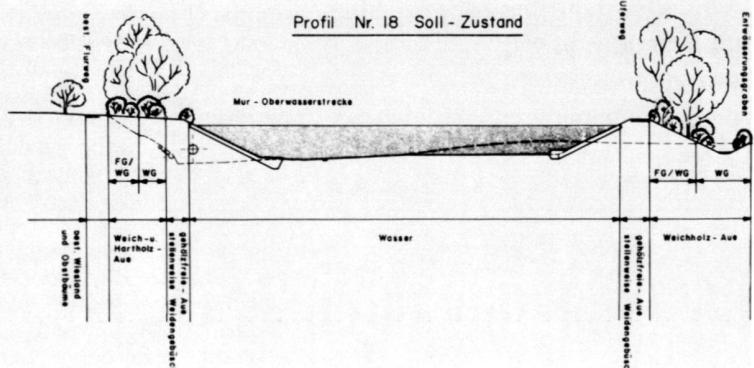
Fig. 3: Existing and planned cross-section of the Mur (diagrammatic).
