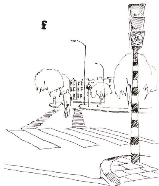
tion can be realized with sidewalks on either side. Oncoming traffic is directed by guiding units and carriageway marking.
