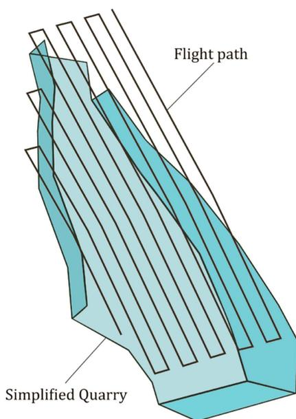
**Figure 4:** Grid pattern flight path with simplified eastern part of the quarry. The distance between drone and track bed was maintained at approximately 20 m. The distance between grid lines was kept at around 8 m. Images were taken approximately every 10 m along the flight path.
