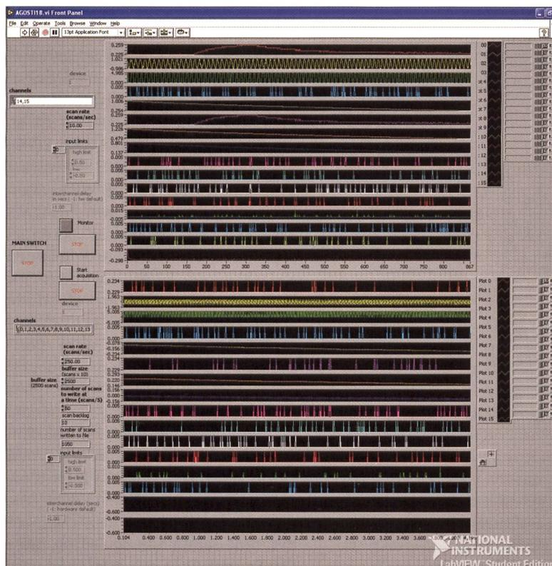
Fig. 3. Front Panel of the fast acquisition system driver in Labview. The 16 upper graphs show pre monitoring of the signals, whereas the lower 16 graphs show visualization during data-acquisition, in which an ASCII text file is first saved, and the data are added until the stop button is activated.
