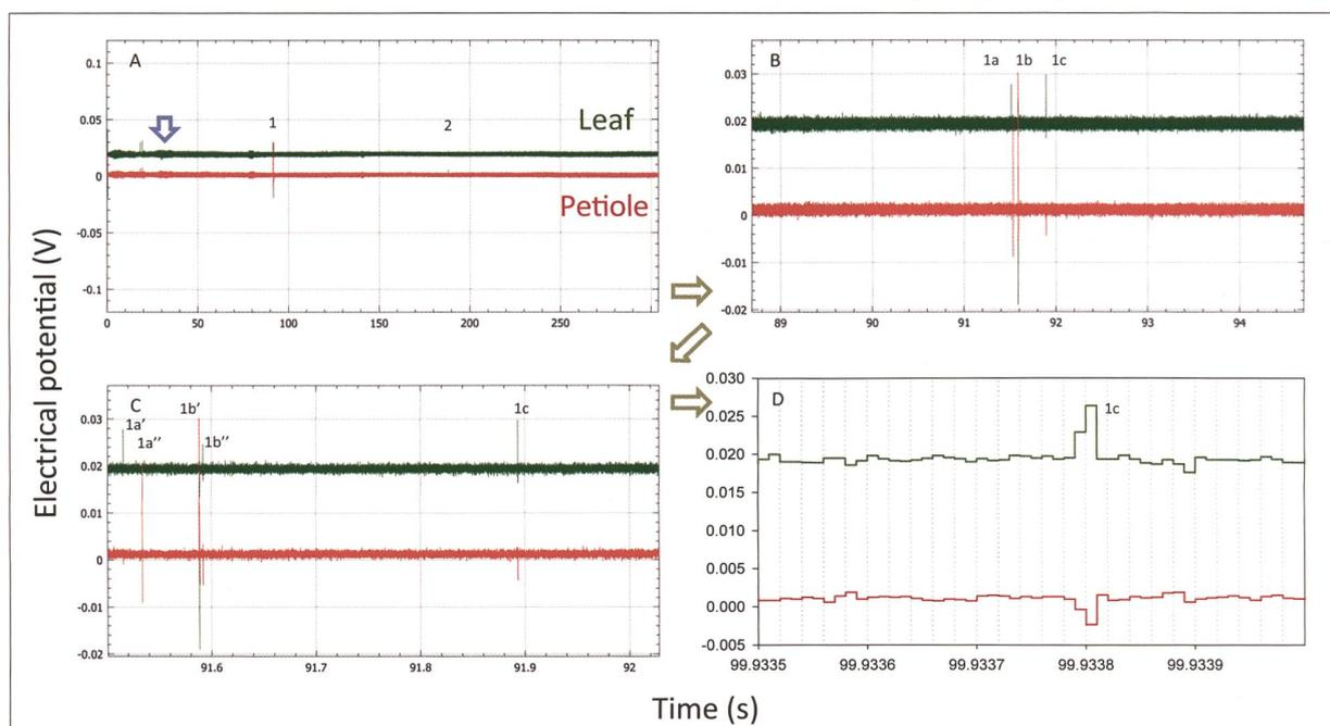
Fig. 6. Recording at 100 000 Ss. Fast events characterization. The results of treatment with a drop of 10  $\mu$ L of water is shown, and time span was successively measured until individual peaks events could be characterized in amplitude, duration, and time shift between leaf and petiole peaks.
