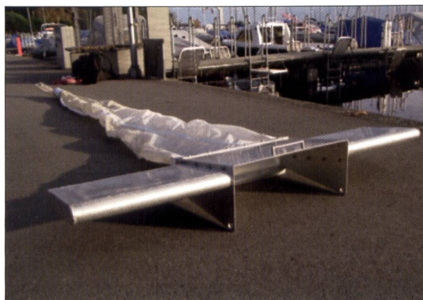
Fig. 1. The Manta trawl used to sample microplastics. Equipped with a 300 \mu m sieve, its mouth is 60 cm wide and dips 25 cm into the water. Picture: Vasco Neuhaus.
