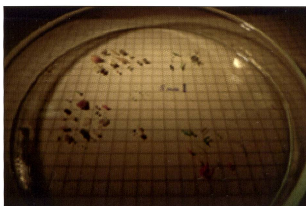
Fig. 4. Microplastics found in Lake Geneva using the Manta trawl.
