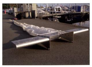
Fig. 1. The Manta trawl used to sample microplastics. Equipped with a 300 µm sieve, its mouth is 60 cm wide and dips 25 cm into the water. Picture: Vasco Neuhaus.
