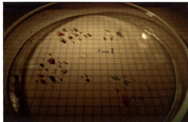
Fig. 4. Microplastics found in Lake Geneva using the Manta trawl.
