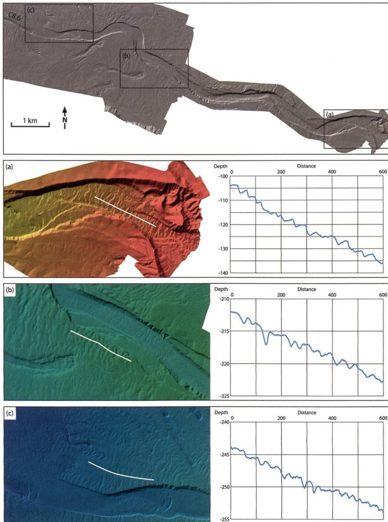
Fig. 9 Depth-distance profiles (m) across bedform fields within and near the main Rhone delta channel (see upper panel for locations). Sand waves with typical wavelengths of  $\sim 50$  m and heights of  $\sim 2$  m occur on the channel floor in the proximal-central part (a). Slightly smaller sand waves characterize the areas on the sides of the main channel in a more distal part (b, c). White lines on the bathymetry maps locate depth profiles.
