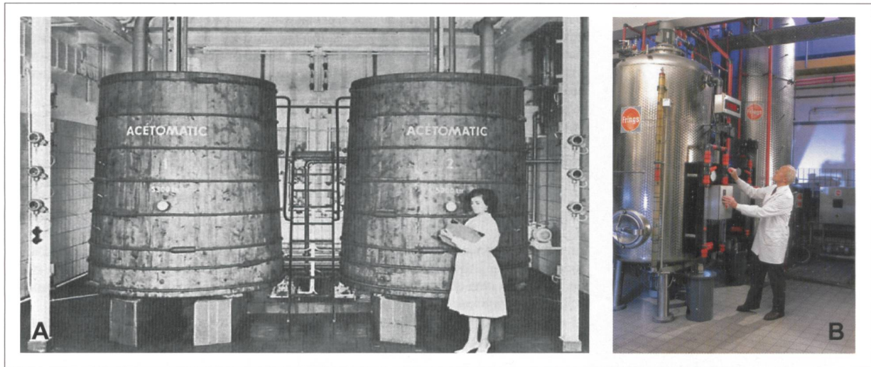
Fig. 10: Submerged acetification systems.
