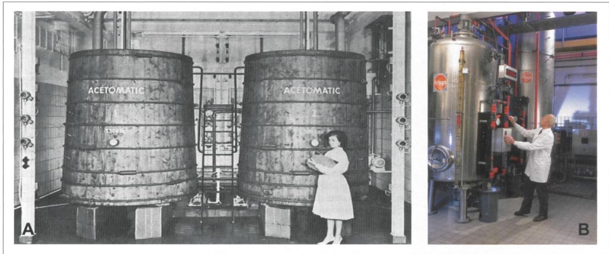
Fig. 10: Submerged acetification systems.
