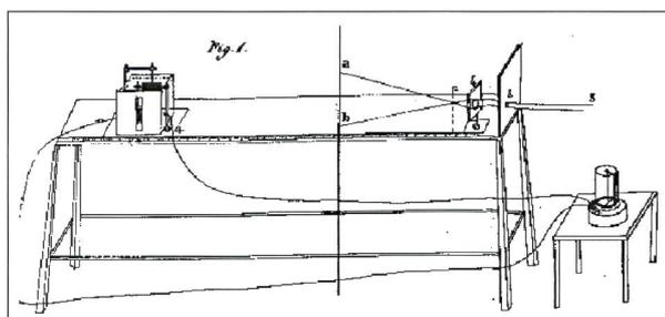
Fig. 5. Electrochemical actinometer (original engraving).
