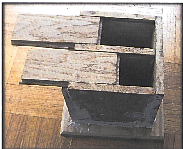
Fig. 8. Top of the tank, hatches and partition.
