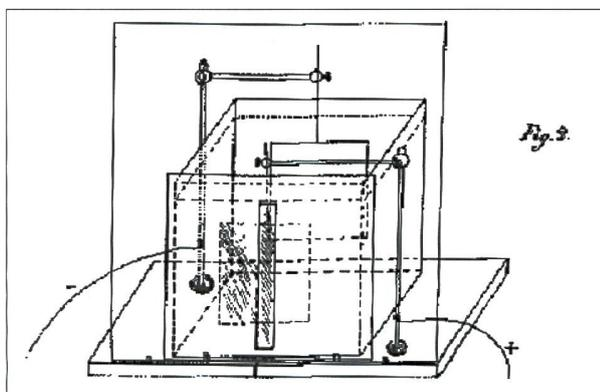
Fig. 4. Electrochemical actinometer wooden box (original engraving).
