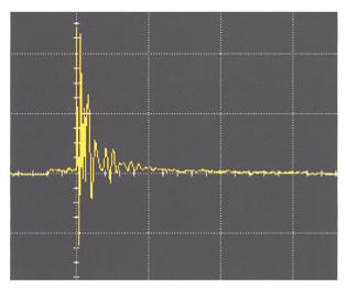
Fig. 5. Oscilloscope screen trace of voltage in time, induced in the spiral when current stops due to breaking connection from liquid metal. Vertical: 200V/div; Horizontal: 5us/division.
