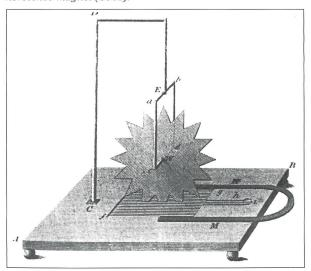
spiral allowed for looking into what went on along differing electrical paths inside the turns. Page took advantage of this flexibility by trying out novel paths running through the spiral and the external apparatus. By contrast, with Henry's spiral and Davis' commercial one, experimental access was limited to the one path running between the inner and outer termini.
