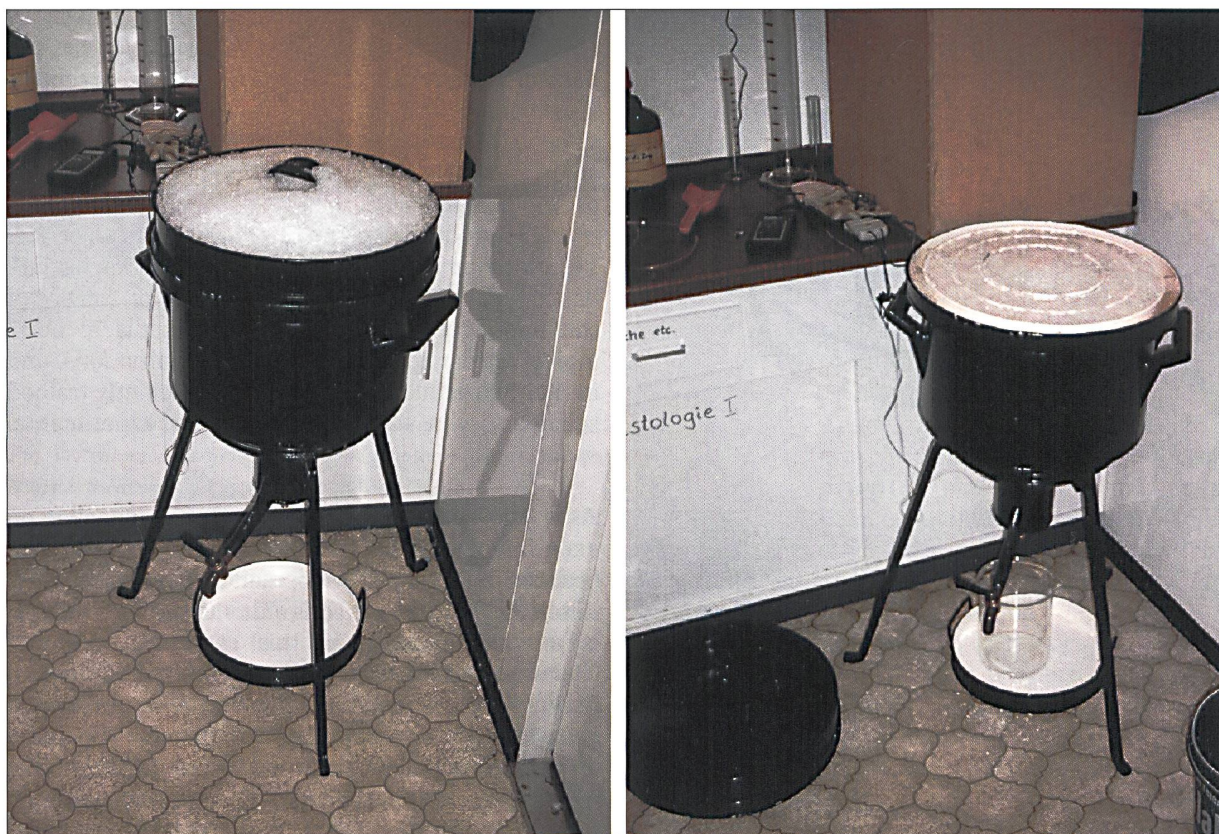
Fig. 14. The ice calorimeter in the cooling chamber. Photo: U. Drüding.
