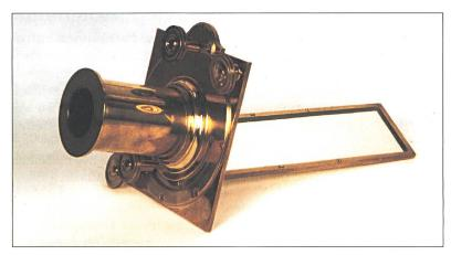
Fig. 17. The reconstructed helioscope. Photo: W. Knust, Museum für Mensch & Natur.
