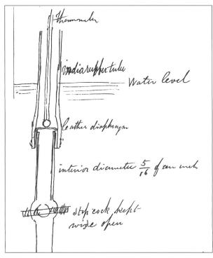
Fig. 13. Joule's drawing of the porous plug.
