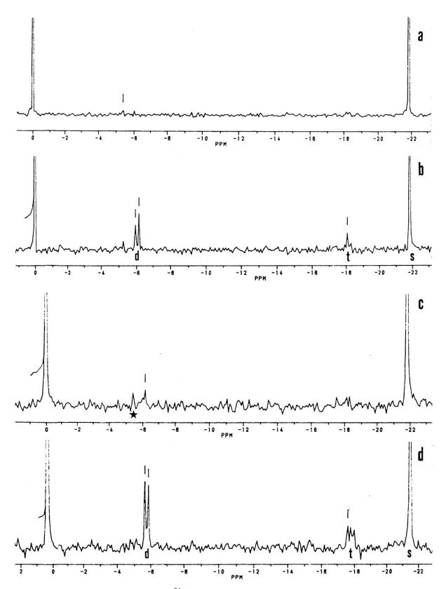
Fig. 1C. Comparative intensities of the  $^{31}P$  NMR spectral signals of linear triphosphate (doublet = d + triplet = t) increasingly decyclized (11-18 days) from 5 mM trimetaphosphate (singlet = s) by 10 mM Mg<sup>2+</sup> ions alone (a,c) and decyclized by nucleophilic attack of the pyrimidine **uracil** (5 mM) doped by 10 mM Mg<sup>2+</sup> ions (b,d).
