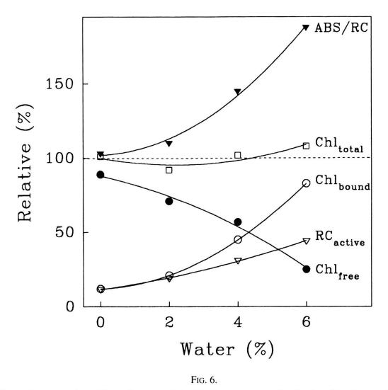
Effect of water on bound/free pigments of thylakoid membranes after 5 min of incubation in HTS reverse micelles. The role of water on the % of active RC and ABS/RC is also shown (see Table 1 for details).
