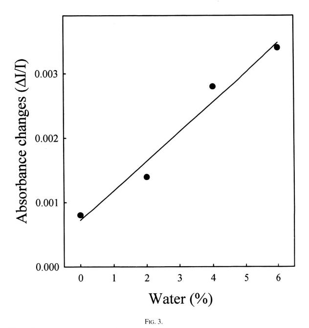
Effect of water on photooxidation of the reaction center, P, measured as light induced absorption changes after 1 hr of incubation in HTS-reverse micelles with different amount of water.
