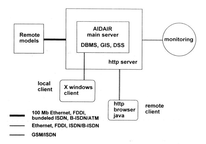
Fig. 6. EUREKA client server architecture diagram.
