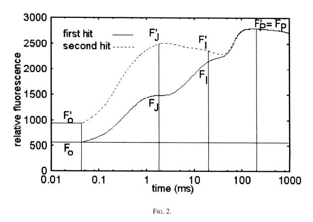
The fast phase of chlorophyll a fluorescence induction in plants: first illumination (first hit) of dark adapted plants, and second illumination (second hit) after 10 s of darkness. Experimental data obtained with a shutter-less system (Plant Efficiency Analyzer built by Hansatech Ltd.). (Also see /8/).
