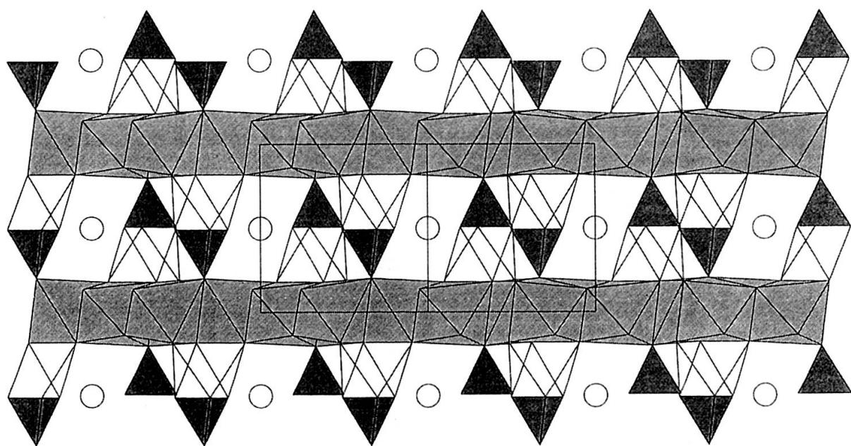
FIG. 2. Projection onto (110) of the atomic structure of schulenbergite showing the brucite-like layers of edge-shared  $\text{CuO}_6$  octahedra which are joined together mostly via the  $\text{SO}_4$  groups and their attached hydrogen bonds.
