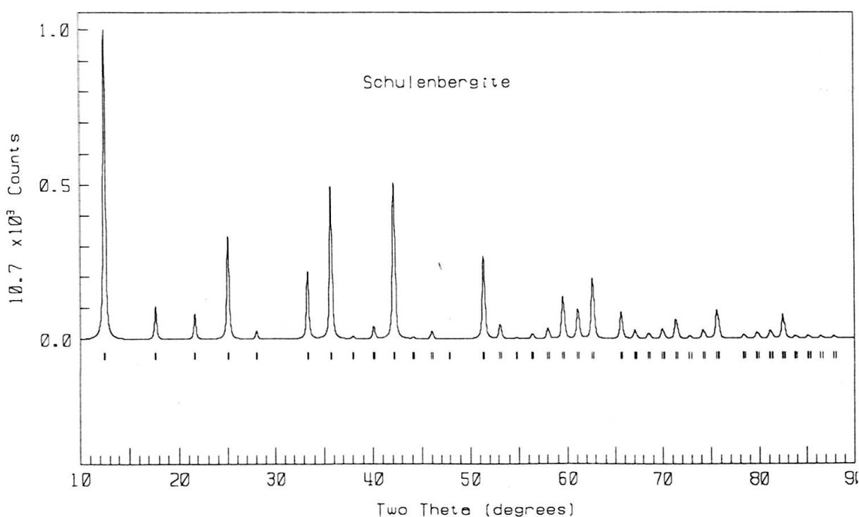
FIG. 3. Calculated powder pattern for Cu-riche schulenbergite.
