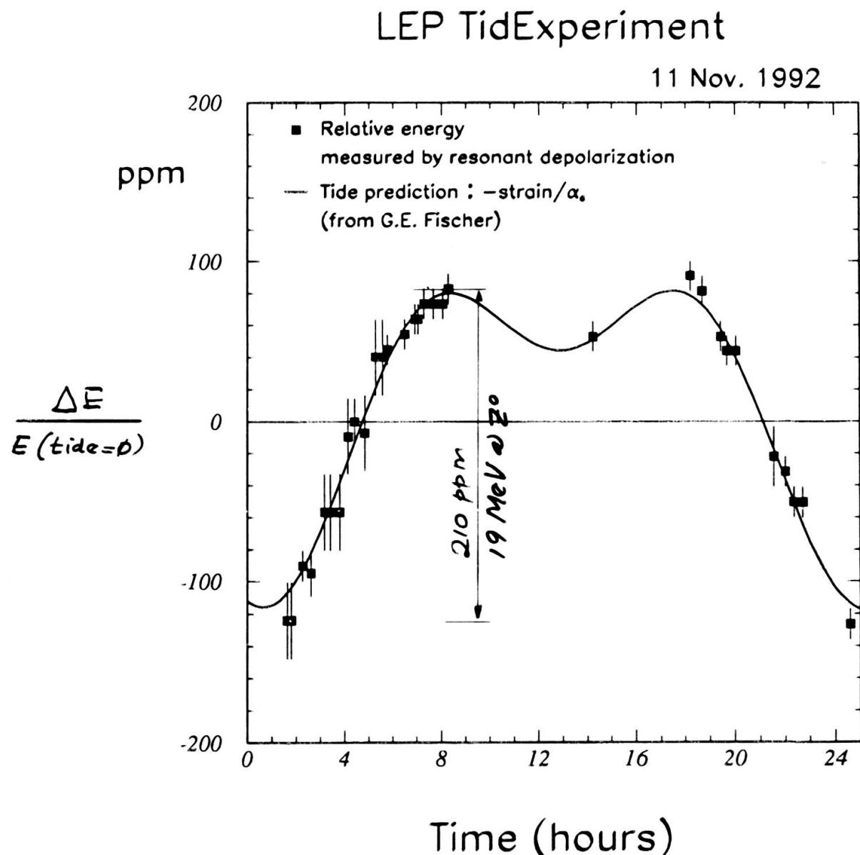
The energy of the electrons and positrons accelerated in the Large Electron-Positron (LEP) collider at CERN depends upon the actual length of the machine, which pulsates according to the tidal motion of the crust of the Earth.
