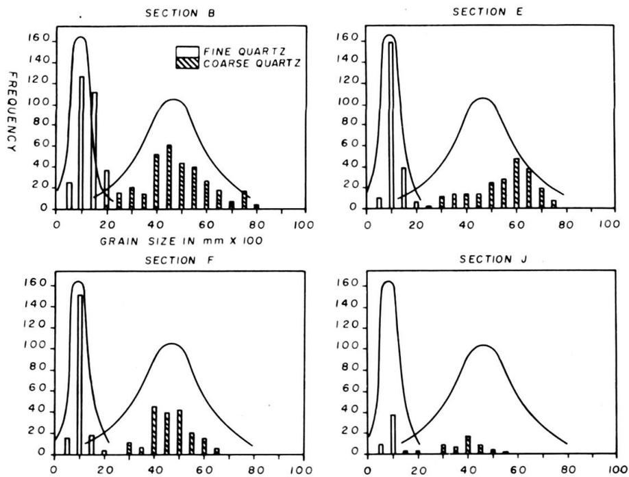
FIG. 7. — Histograms and corresponding theoretical curves showing distribution of bimodal arenites in sections B, E, F, and J.
