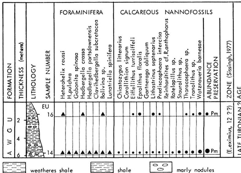
FIG. 3. — Distribution of planktic microfossils in the Awgu Formation exposed in a roadcut on the Enugu-Port Harcourt expressway, 47 km before the expressway — old Umuahia road junction.
