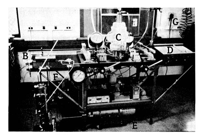
Fig. 1. — Experimental test apparatus. A: circulator; B: pore fluid sampler; C: pressure vessel; D: X-Y recorder; E: intensifier-accumulator; F: gear pump; G: source of CO<sub>2</sub>.
