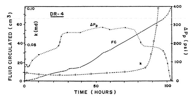
Fig. 7. — Experimental results, test DR-4.
