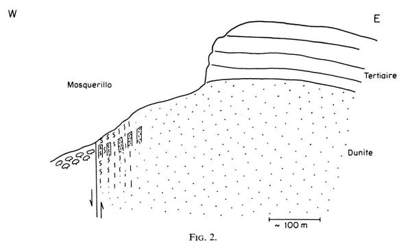
Schematic diagram illustrating the serpentinized band, between phases 5 and 6 (see Fig. 1). The degree of serpentinization and rodingitization diminishes downwards and towards the east
