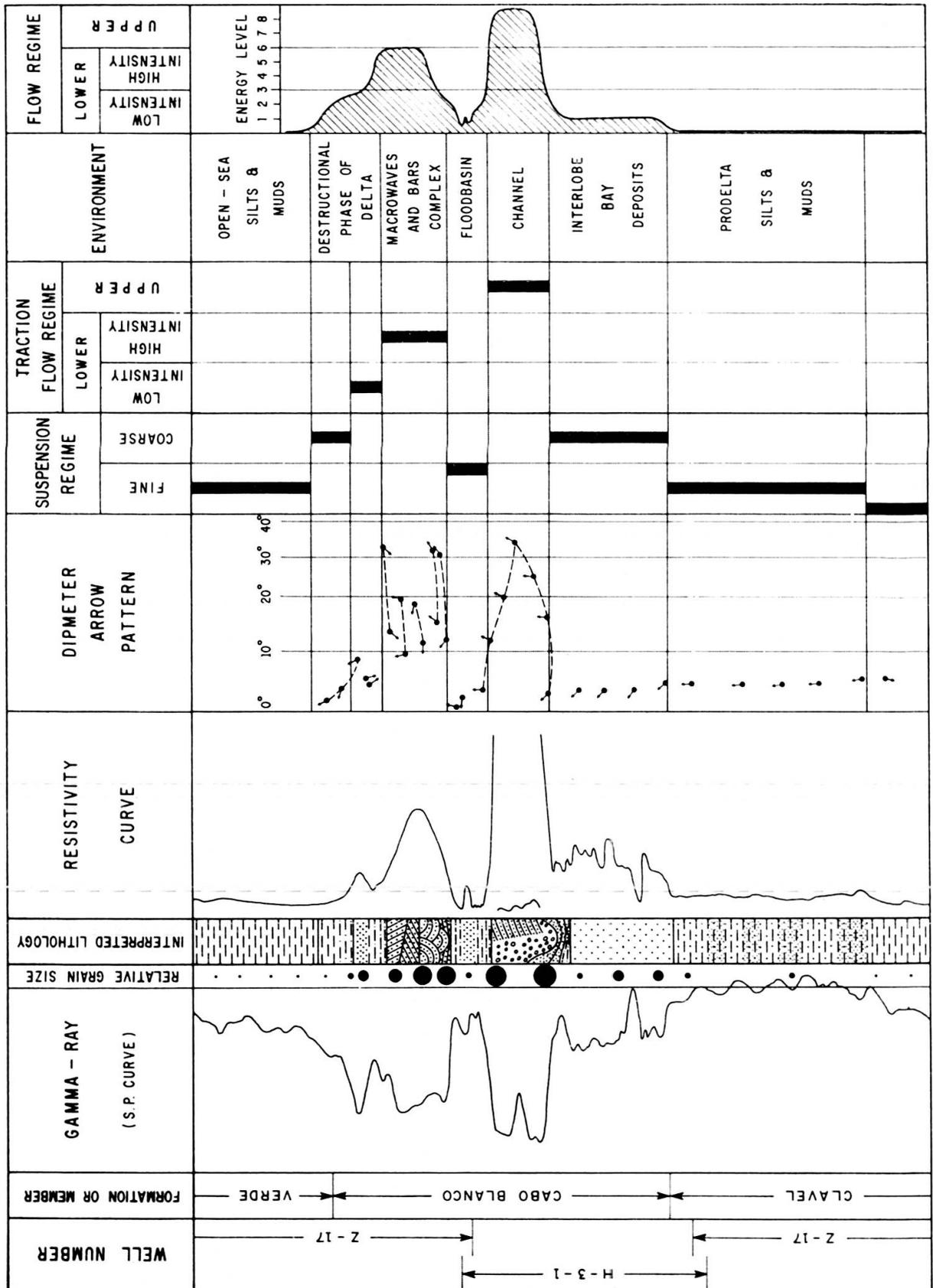
FIG. 13. — Generalized sedimentary-electric composite log of the Cabo Blanco Sandstone.
