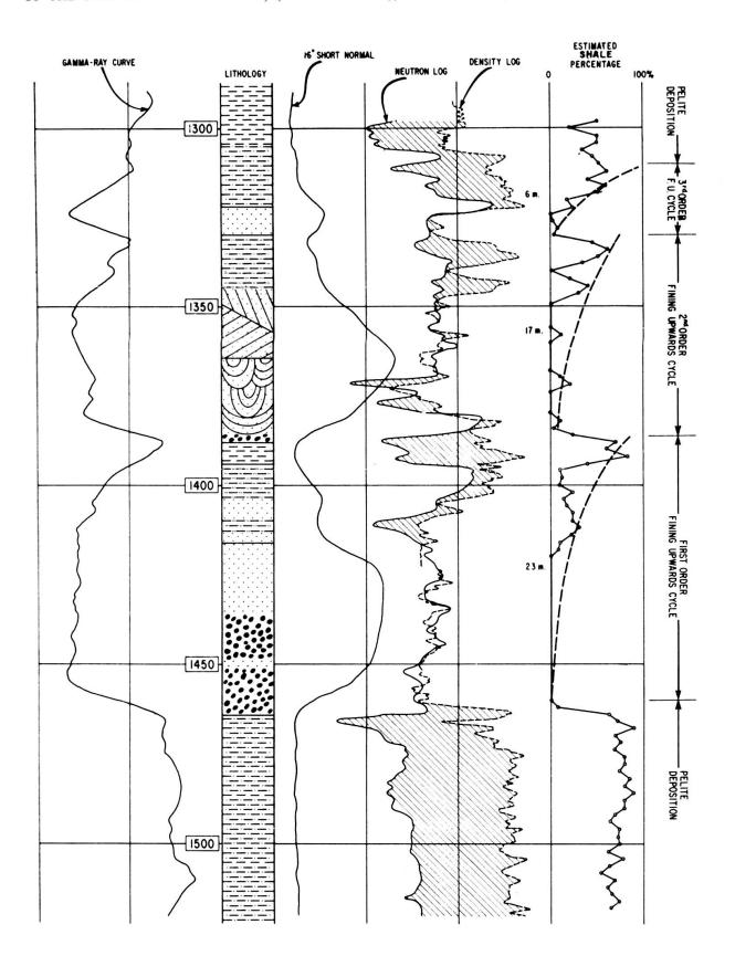
Fig. 9. — Recognition of sedimentary cycles by combination of various types of electric logs.
