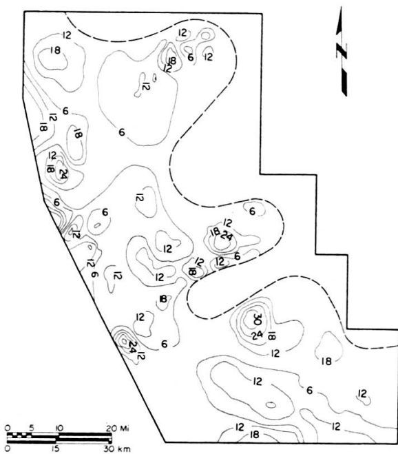
FIG. 15. — Chlorite distribution map (% of total clays).
