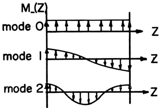
FIG. 9. — The normal modes of oscillation of the spin density in a metallic slab.
