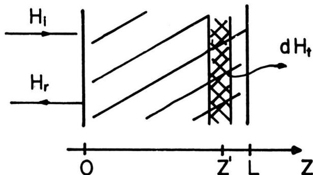
FIG. 3. — The transmitted field is a superposition of fields radiated by the precessing magnetic moments at different points in the metal.
