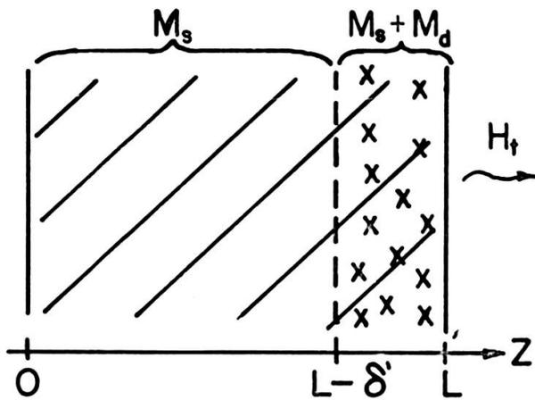
FIG. 4. — Idealized geometry describing ion-implantation experiments.
