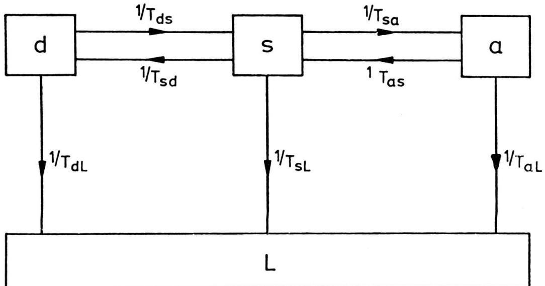
FIG. 1. — Schematic diagram of relaxation processes in bottlenecked  $EPR$ . The primary  $3d$  impurities, the conduction-electron spin magnetization, and the additional  $3d$  impurities are denoted  $d$ ,  $s$  and  $a$  respectively, and the temperature bath ("lattice") is denoted  $L$ .
