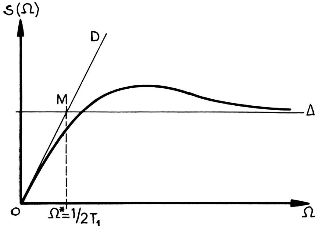
FIG. 1. — Determination of  $T_1$  from the curve  $s(\Omega)$  in the modulation method. The curve  $s(\Omega)$  is plotted by means of the experimental datas. The straight lines  $D$  and  $\Delta$  are deduced of it. The abscissa of  $M$ , the point where  $D$  and  $\Delta$  are crossing, yields  $1/2 T_1$ . For very short  $T_1$ , the beginning of the curve is only traced and gives  $D$ . We find indirectly  $\Delta$  by comparing the signal  $s$  with the transmitted signal  $v$ .
