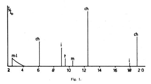
Diffractogramme type anticathode Cu filtre Ni. m-1 = mixed-layer, ch = chlorite, i = illite, t = talc, m = montmorillonite.
