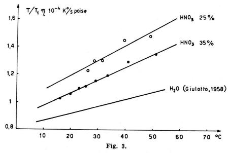
$T/T_1\eta$  versus T for two samples of acqueous solutions of nitric acid.
