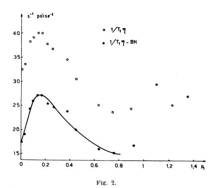
$1/T_1\eta$  and the difference  $1/T_1\eta$  — BN versus  $p_1$  for acqueous solutions of nitric acid.
