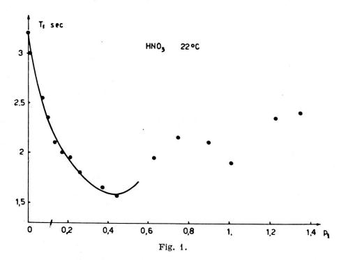
$T_1$  of acqueous solutions of nitric acid versus the proton concentration  $p_1$  in the  $H_3$   $O^+$  group. This quantity is related to the molar fraction of acid  $N_1$  by the relationship  $p_1 = 3N_1/(2-N_1)$ .
