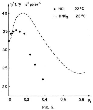
$1/T_1\eta$  versus  $p_1$  for acqueous solutions of hydrocloric acid. The dashed curve is the corresponding curve for  $HNO_3$ .
