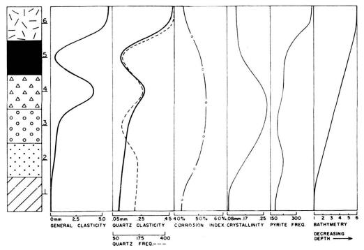
COLUMN SHOWING PARAMETER VARIATIONS OF MICROFACIES — SECTION I Fig. 10  ${\rm Variation\ des\ paramètres\ dans\ le\ cycle\ id\'eal}.$
