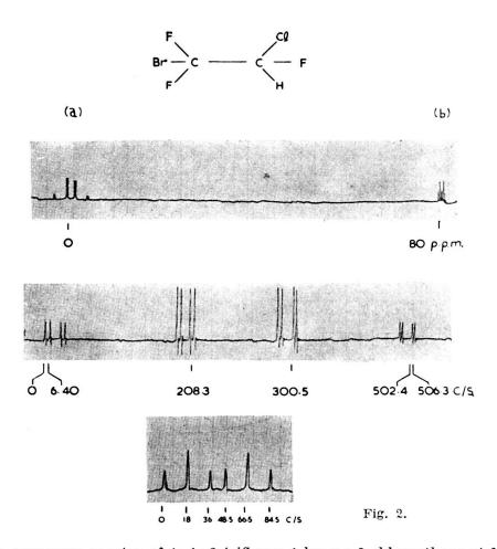
Fluorine resonance spectra of 1:1:2-trifluoro 1-bromo 2-chloroethane at 60 Mc/s, (a) CF<sub>2</sub> Br group and (b) CFClH group.
