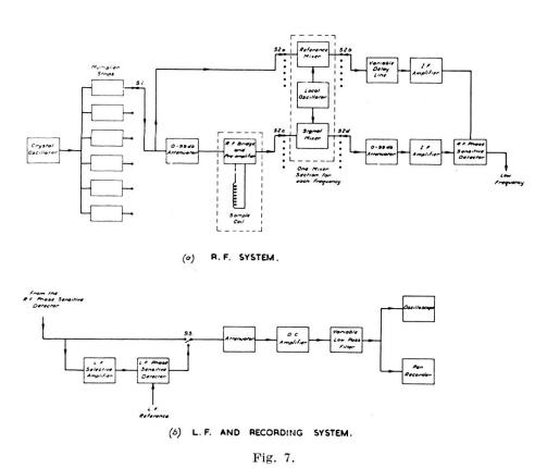
Block diagram of the r.f. and the l.f. sections.
