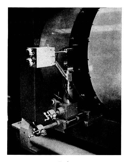
Fig. 3. The probe and moving mechanism of the R.S.2 withdrawn from the magnet gap.
