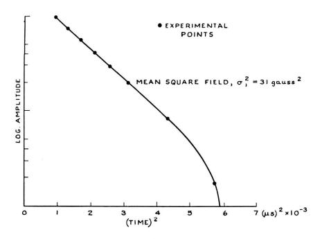
FIG. 2. AMPLITUDE OF INDUCTION DECAY, FROM <sup>51</sup>V NUCLEI IN VANADIUM METAL, AGAINST (TIME)<sup>2</sup>
