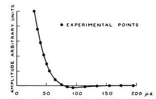
FIG.1. INDUCTION DECAY, AFTER  $\frac{\Pi}{2}$  PULSE, FROM TRANSVERSE NUCLEAR MAGNETIC MOMENT OF  $^{5\,\mathrm{I}}$  V NUCLEI IN VANADIUM METAL.
