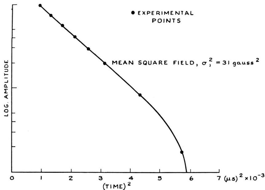
FIG. 2. AMPLITUDE OF INDUCTION DECAY, FROM  $^{51}\text{V}$  NUCLEI IN VANADIUM METAL, AGAINST  $(\text{TIME})^2$
