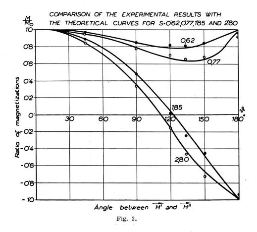
lation of the magnetic field. After the battery of condensers was discharged and the water with the changed magnetization passed through the resonance coil, the change of the amplitude of resonance lines was observed. For H'' > H' and for sufficiently large angles  $\theta$  the lines were reversed. The maximal effect on each record depends on the ratio  $M/M_0$  and on the degree, to which the tube in the region of the resonance coil is filled by water with
