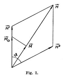
on the suitable choose of the series resistance. The angle  $\theta$  between H' and H" could be changed by rotating the loop. As the field H" was set in a fraction of a microsecond the transition was nonadiabatic one. All other transitions i.e. the decay of H" and the entry of water into the strong field of the electromagnet took place sufficiently slowly to fulfil the condition of adiabatic passages.
