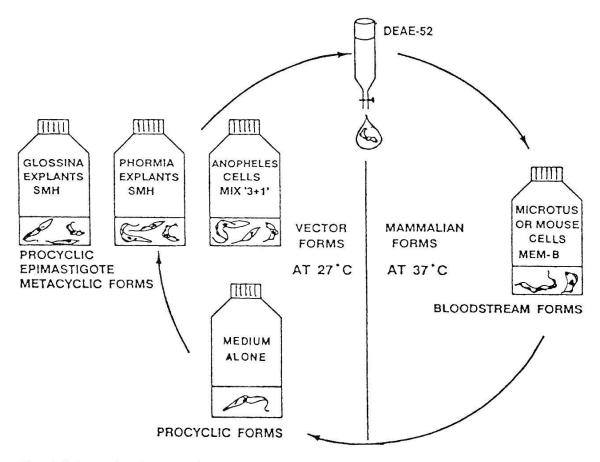
Fig. 6. Schematic diagram of the culture systems.
