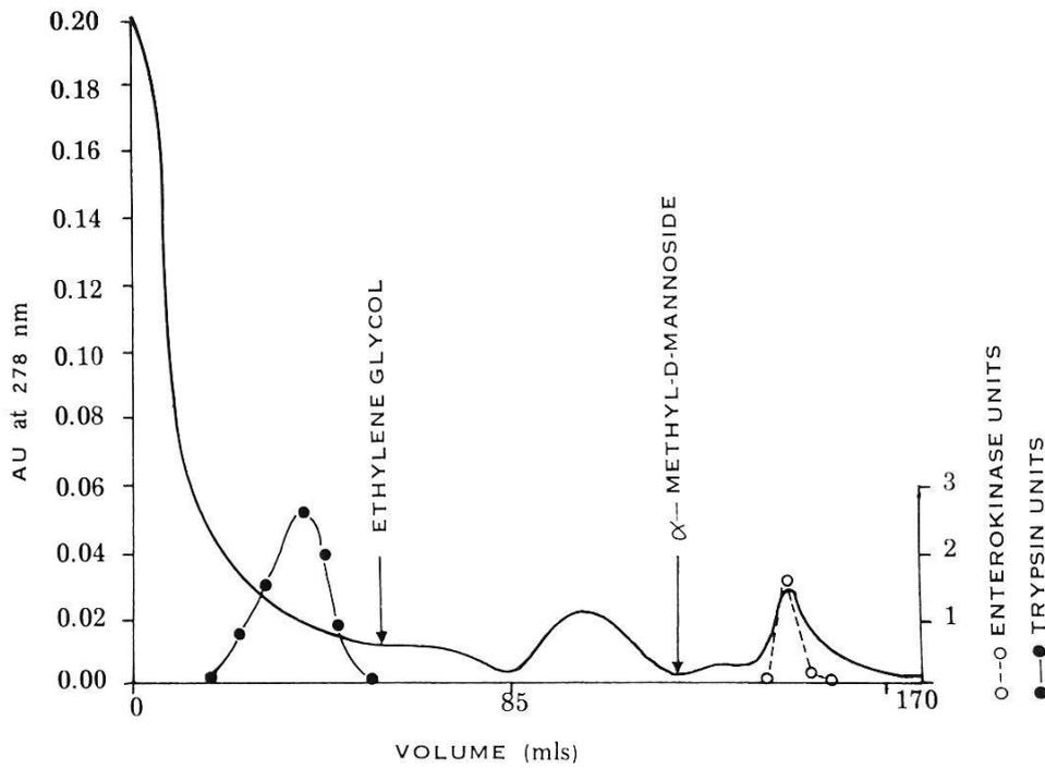
Fig. 4. Separation of *G. m. morsitans* gut enterokinase by affinity chromatography on concanavalin A-sepharose 4B. Flow rate,  $15 \text{ ml} \cdot \text{h}^{-1}$ . Enzyme activities expressed in  $\mu\text{moles} \cdot \text{min}^{-1} \cdot \text{ml}^{-1}$ .
