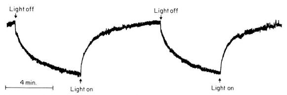
Fig. 5. Continuous record of the changes in the ESR signal amplitude of the rose bengal radical during illumination at the field position of maximum displacement of the derivative signal.
