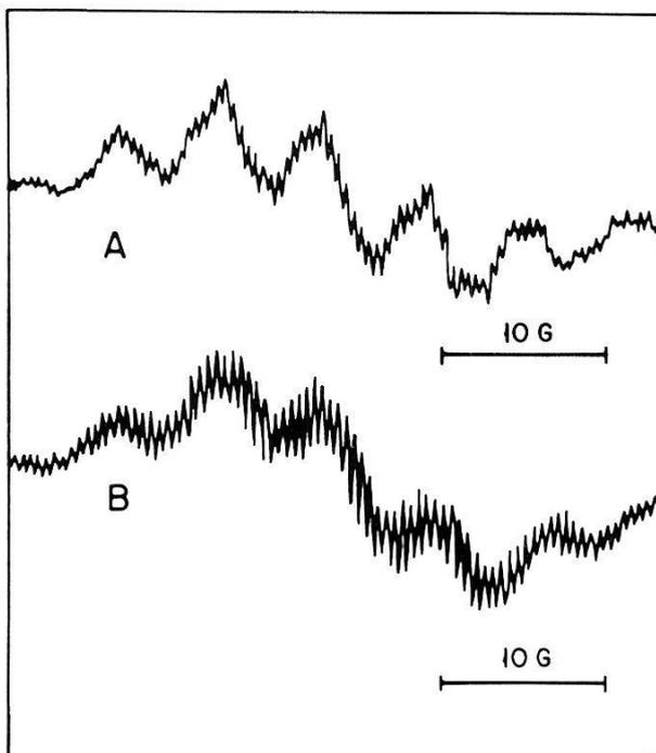
Fig. 2. X-Band (3 cm) ESR spectra of phenazine methosulfate free radical: (A) Recorded 50 min after the mixture of the *T. cruzi* epimastigote suspension and PMS. The spectrum was recorded at 0.66 gauss/min, the modulation amplitude was 0.16 gauss at a frequency of 100 KHz. (B) Same spectrum recorded at 2.50 gauss/min showing a better resolution of the signal.
