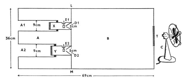
Fig. 1. Gouck's type of olfactometer.
