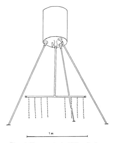
Figure 6. The apparatus for DDT application.
